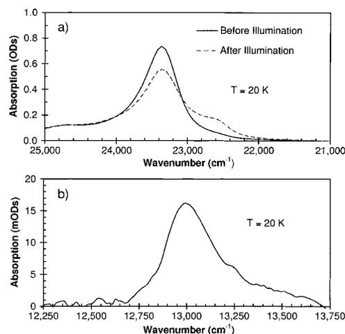
**Figure 1.** (a) The Soret spectrum of the intermediate state at 20 K before and after illumination with a laser diode. Absorption from [Ru(bpy)<sub>3</sub>]<sup>2+</sup> has been subtracted to more clearly demonstrate the changes in the Soret region. The sperm whale Mb concentration was 5 mM. (b) The difference spectrum from before and after illumination measured in the near-IR using a 17 mM sperm whale Mb sample.
